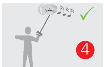
Press the user key for approx. **5 seconds**. If the **test alarm** sounds (1 sec. on / 1 sec. off), the **smoke alarm is in working order**.
